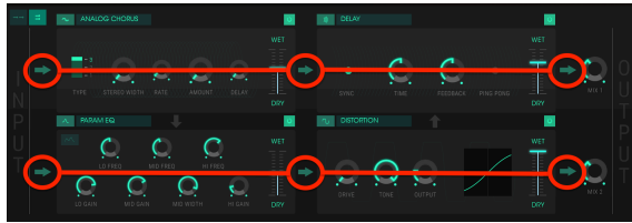
Signal flow of the FX chain in parallel mode
