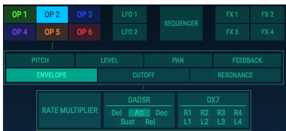
Selecting the DADSR envelope attack for Operator 2 as a mod destination
